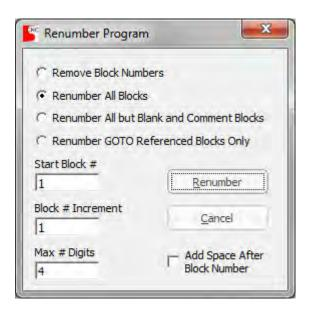
This dialog allows you to set up how you would like your program blocks to be numbered. The *Start Block #*, *Block # Increment* and *Max # Digits* settings define how the program will be numbered.
