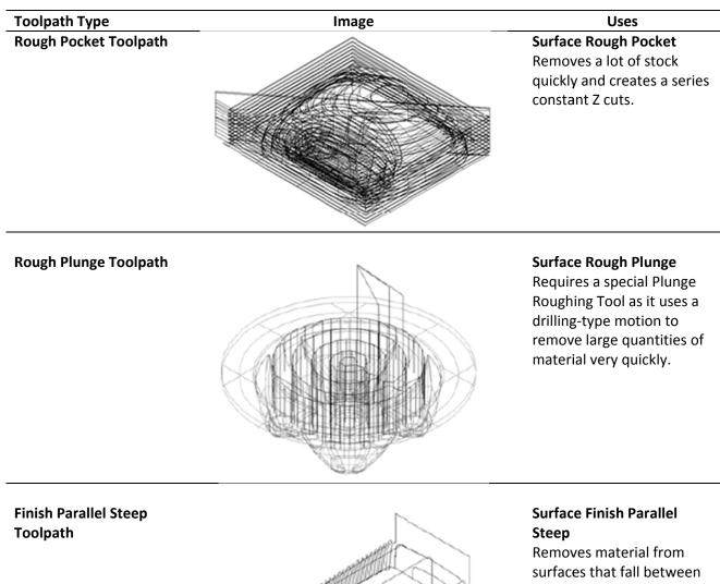
surfaces that fall between two slope angles. This toolpath is usually used after a finish parallel toolpath.
