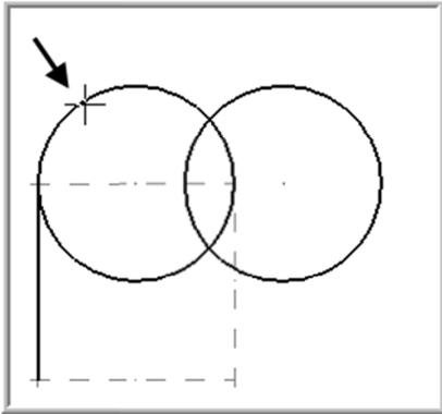
23. To satisfy the prompt **Specify the second endpoint** move the cursor over the area of the circle shown below. Ensure there is **no visual cue** being displayed and click on this point. As **Tangent** is activated on the line ribbon bar the line will snap to the closest tangency point on the circle as shown below right.
