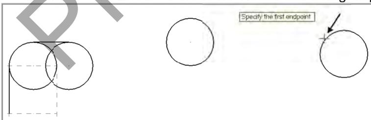
26. To satisfy the prompt **Specify the second endpoint** move the cursor over the area of the circle shown below. Ensure there is **no visual cue** being displayed and click on this point. As **Tangent** is activated on the line ribbon bar the line will snap to the closest tangency point on the circle.
