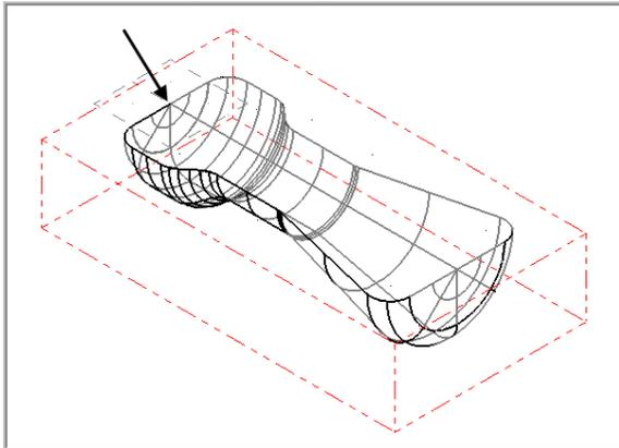
Surface roughing toolpaths typically use larger tools, multiple stepovers, and multiple step downs to quickly remove larger volumes of stock and leave an even amount of stock for finishing.
